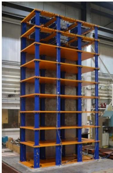
**Figure 1. 9 story test structure**
